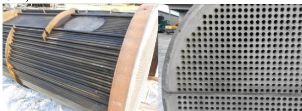
Figure 3. C105A Before cleaning
