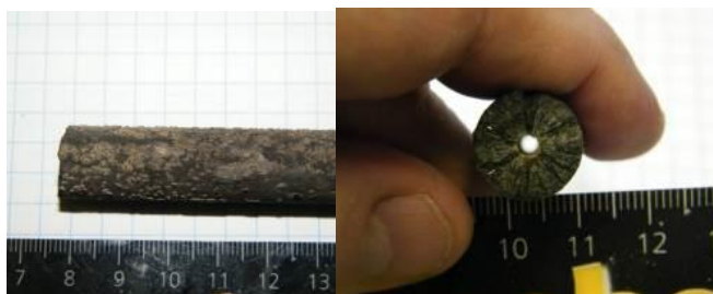
Figure 2. Samples of crystalline deposit ( \text{FeCO}_3 ) removed from a tube side from Lean-Rich amine exchanger.
